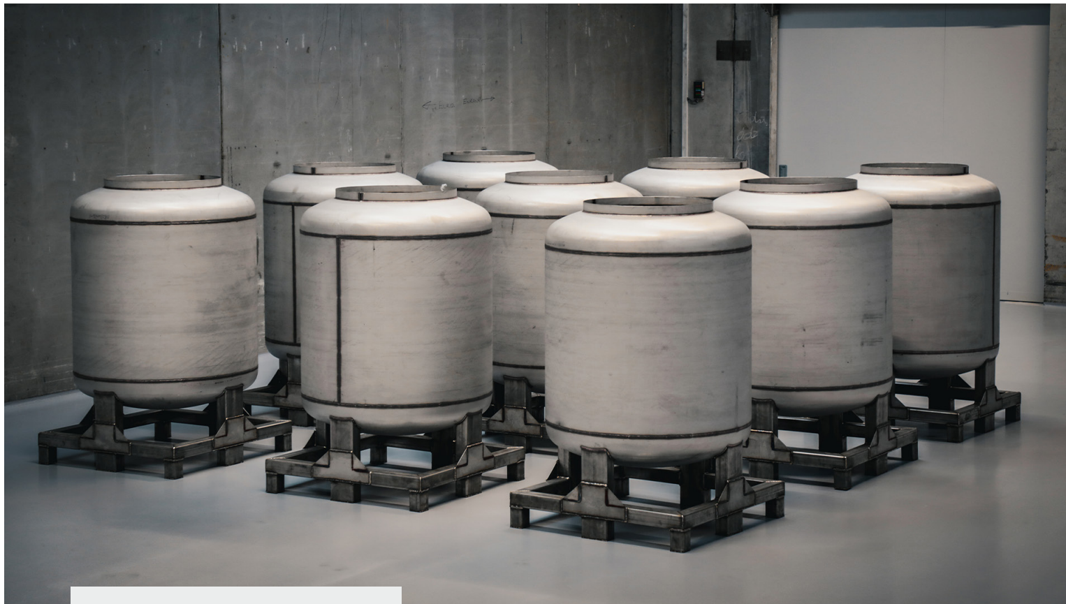
Figure 6. Tanks for tonne scale molten salt production and transportation. Each tank holds 1 cubic meter of salt.
