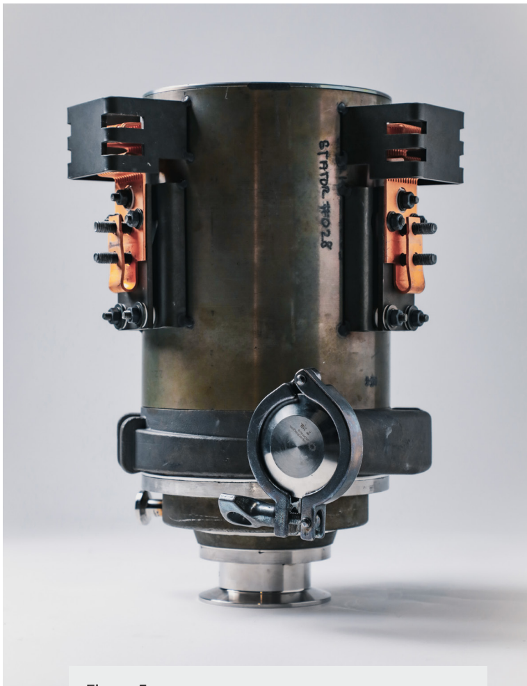
Figure 5. Left: the small pump with hydrodynamic Bearings. Right: the first version of the AMB pump.
