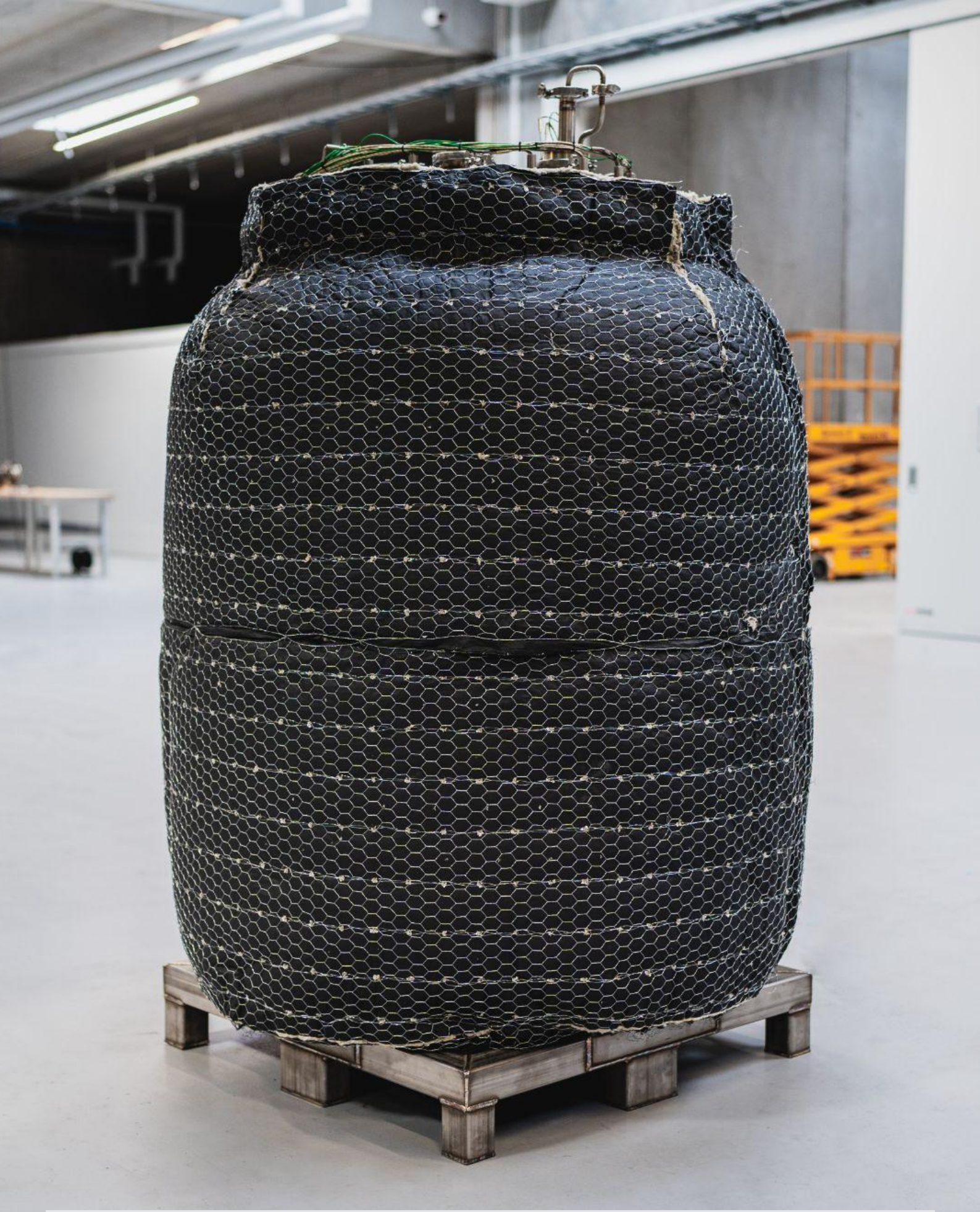
Photo showing version 3.1 transport tank. Version 3.2 will have stainless steel box shroud around the insulation.
